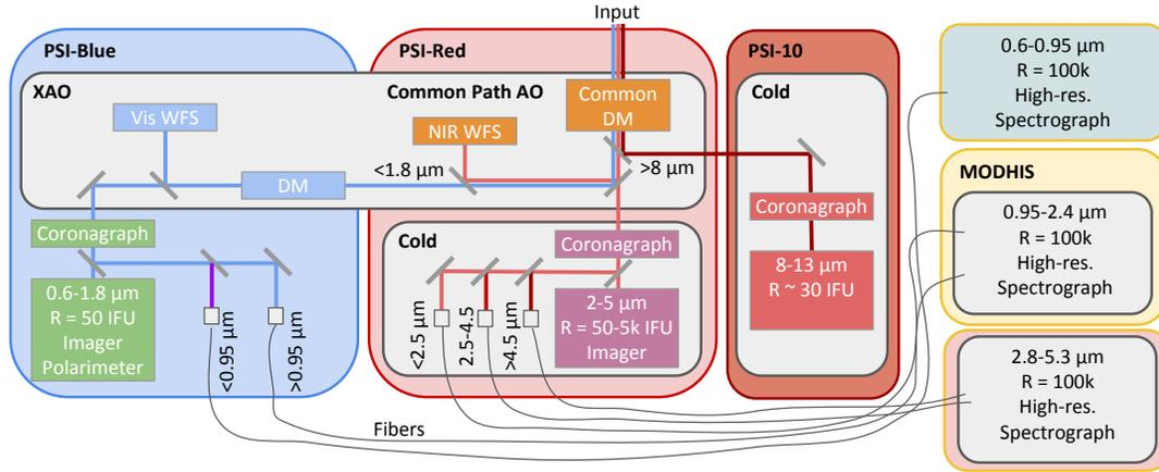
**Figure 3.** Conceptual layout of the PSI architecture. Not shown are atmospheric dispersion correctors and low-order wavefront sensors, as well as the coronagraphic IFS on the 10- $\mu\text{m}$  channel.
