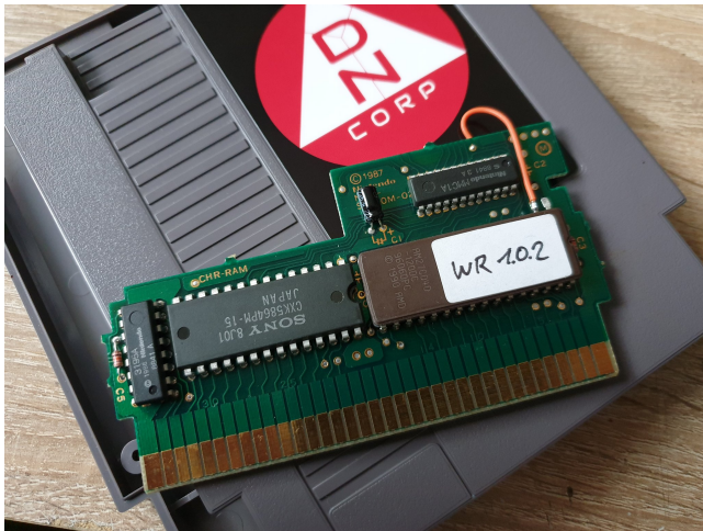
Figure 4: A cartridge of the game What Remains, made by player mi213 by repurposing an old game, and following the project DIY instructions. Photography, mi213, 2021.
