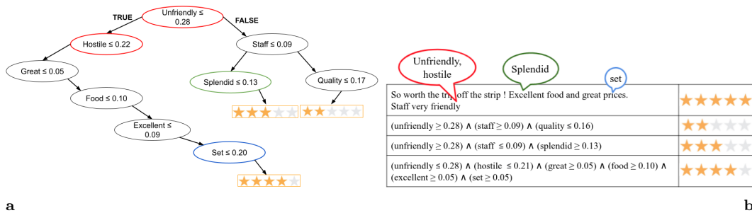
Figure 2. (a) A local surrogate tree explaining CNN1D for a Yelp review. Due to the space limitation, some parts of the original tree are not shown. (b) Decision rules extracted from the tree. The first row of the table shows the document under analysis and its label (five-star review), and the callouts at the top of each word present words from the semantic set (green for synonyms, RED for antonyms, and blue for hyponyms and hypernyms) that was replaced with the word . The second to fourth row are the decision rules extracted from the decision tree and the final labels that are assigned to these rules. The antecedent of rules are in the left column, and their consequents are in the right column.
